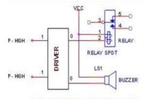
Make Pins High - Relay/Buzzer ON
