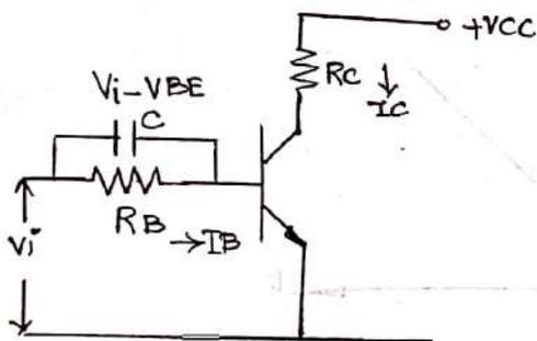
From the dia, the capacitor C is called speed-up or commutating capacitor.
