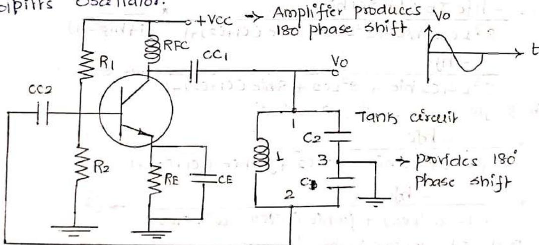
The amplifier stage produces  $180^\circ$  phase shift and tank circuit gives an additional phase shift of  $180^\circ$  to satisfy the oscillation conditions.
