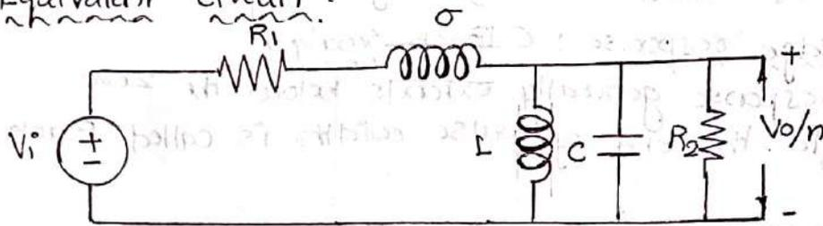
Equivalent circuit of pulse transformer.
