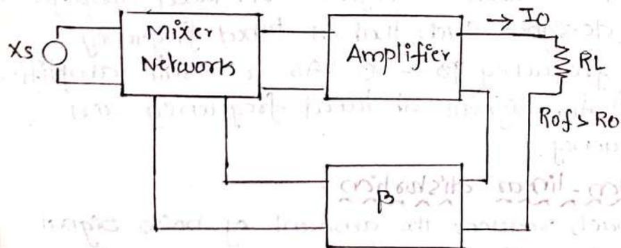
The dia. 2 Shows the negative feedback which samples the output current, regardless of how
