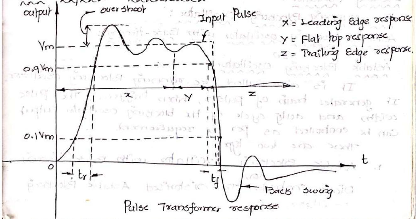
The distorted output response of a pulse transformer is shown above.
