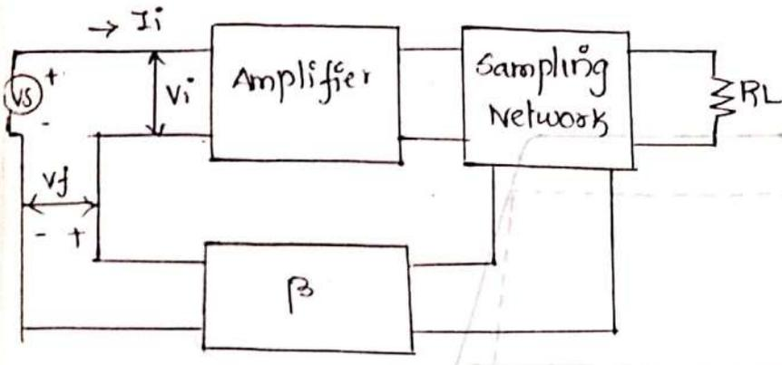
If the feedback signal is added to the input in series with the applied voltage, it increases the input resistance.
