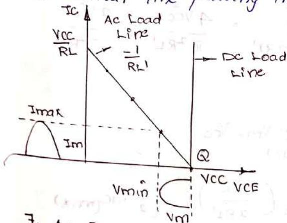
The slope of the ac load line is represented in terms of  $V_m$  and  $I_m$  as
