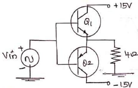
Soln Given  $V_{cc} = 15V$ ,  $R_L = 4\Omega$
