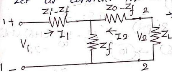
$$\rightarrow Y_T = \frac{I_2}{V_1} = \frac{I_2}{I_1 Z_{11}} = \frac{A_i}{Z_{11}} \rightarrow (2)$$
