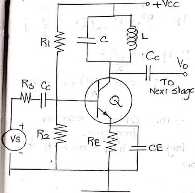
The dia. shows single tuned CE amplifier. Single tuned amplifier circuit uses one parallel tuned circuit as a load in each stage with tuned circuits in all stage tuned to the same frequency.
