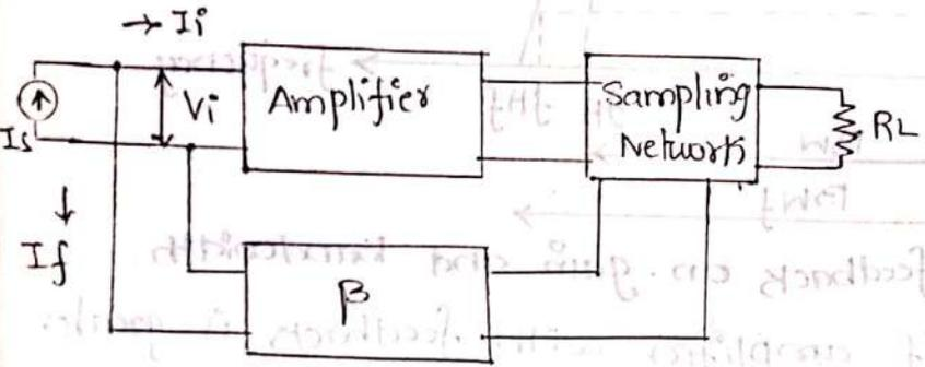
The dia. 2. Shows the feedback signal is added to the input in shunt with the applied voltage, it decreases the input resistance.
