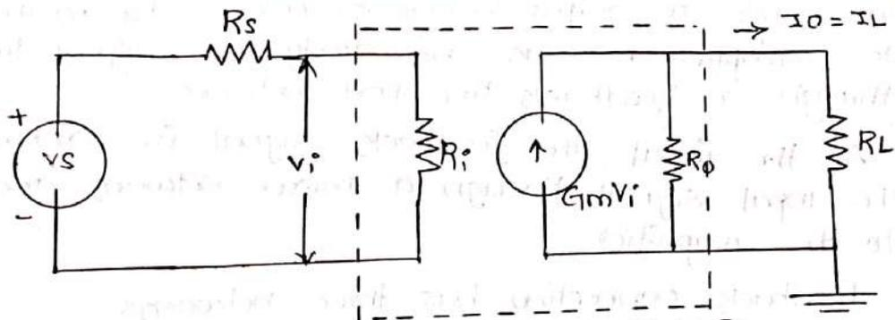
The output current is proportional to the input signal voltage and the proportionality factor is independent of the magnitude of the source and load resistances.
