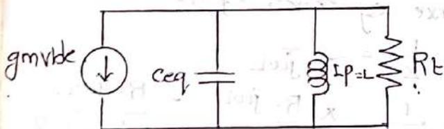
$$\therefore R_t = R_o \parallel R_p \parallel R_i$$
