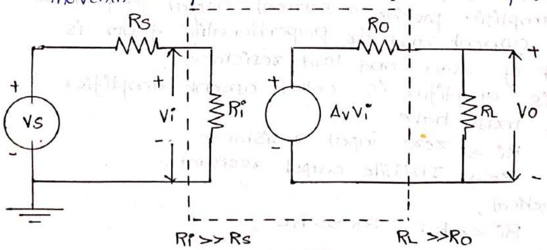
Amplifier input resistance is large compared with the source resistance ( $R_i > R_s$ )
