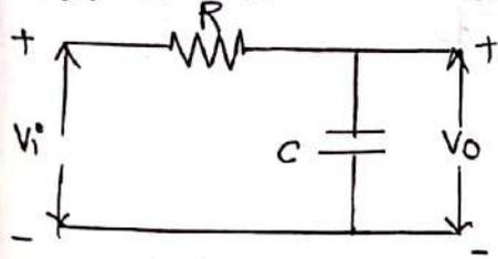
The dia. shows low pass RC. At high frequencies, the capacitor acts as a virtual short circuit and hence output falls to zero. The circuit passes the low frequency readily, hence called low pass RC circuit.
