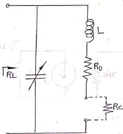
From the circuit, L and C represents tank circuit. The internal circuit losses of inductor are represented by  $R_o$  and  $R_c$  represents the coupled in load.
