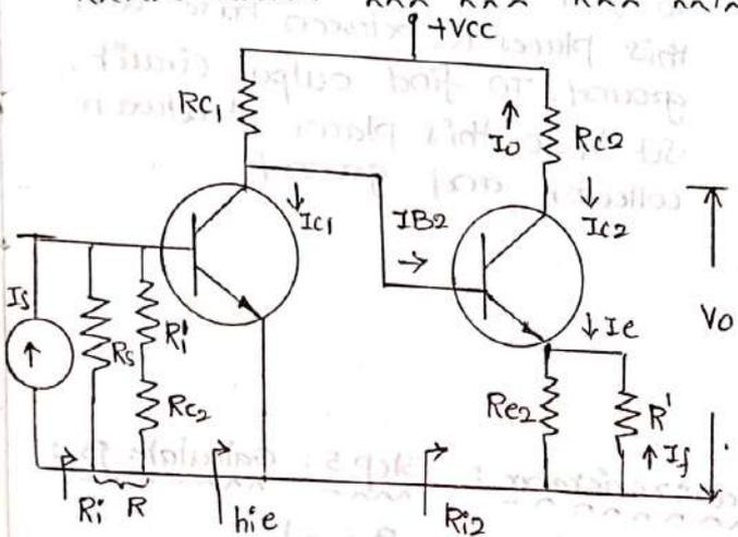
The input circuit without feedback is obtained by opening the output loop at the emitter of  $Q_2$  ( $I_o=0$ ). This places  $R_f$  in series with  $R_{e2}$  from base to emitter of  $Q_1$ . The output circuit is found by shorting the input node (base of  $Q_1$ ) i.e. making  $V_{ii}=0$ . This places  $R_f$  in parallel with  $R_{e1}$ .
