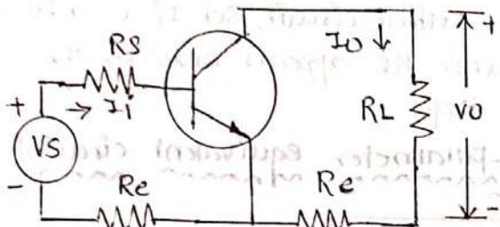
To find input circuit set  $I_o = 0$  then  $R_e$  appears at the input side.
