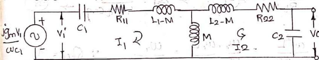
The dia. shows double Tuned RF amplifier in CE configuration. Here voltage developed across tuned circuits is coupled inductively to another tuned circuit.
