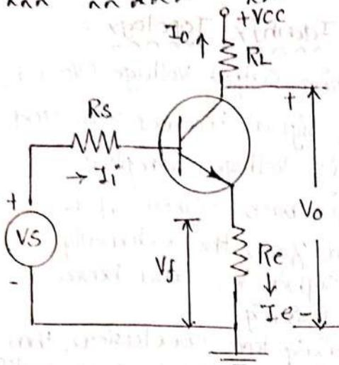
For  $I_o = 0$ , collector circuit is open circuited.
