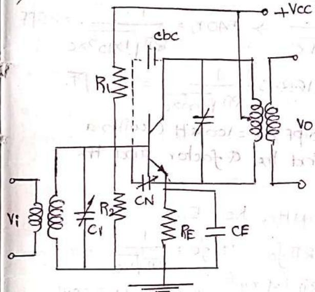
Neutralization using coil:
