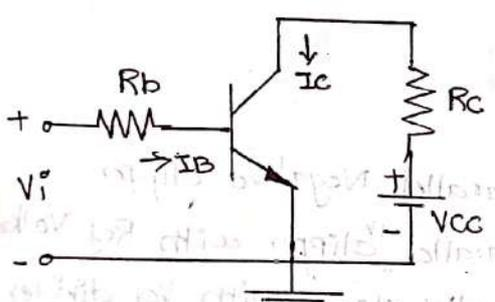
Transistor switching circuit.
