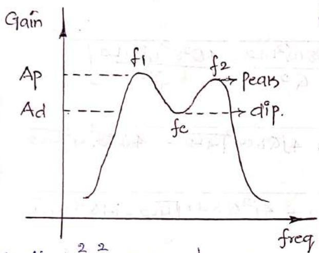
Two Gain peaks of frequency response in double Tuned Amplifier is
