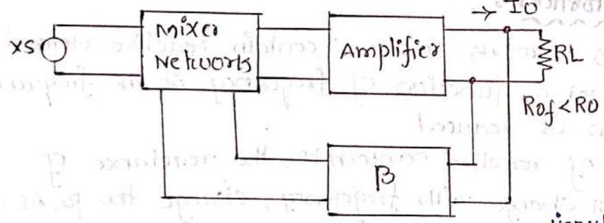
The negative feedback which samples the output voltage, regardless of how the output signal is returned to the input, tends to decrease the output resistance.
