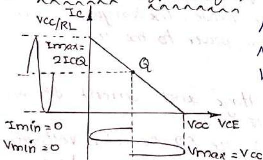
For Maximum Efficiency, Assume maximum and minimum output voltage and current are
