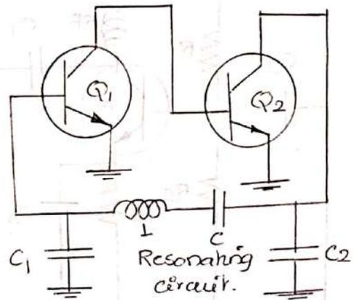
Parallel Resonating circuit  $\rightarrow$  isolation from the active device by using the capacitor  $C_1$  and  $C_2$ .
