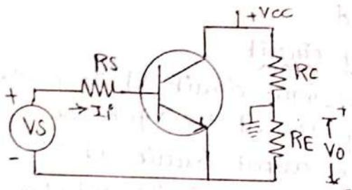
To find input circuit, set  $V_o = 0$ , and hence  $V_s$  in series with  $R_s$  appears between B and E.
