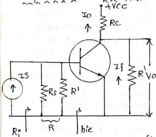
To find input circuit, set  $V_o = 0$ , this places  $R'$  between base and ground. To find output circuit, set  $V_i = 0$ , this places  $R'$  between collector and ground.
