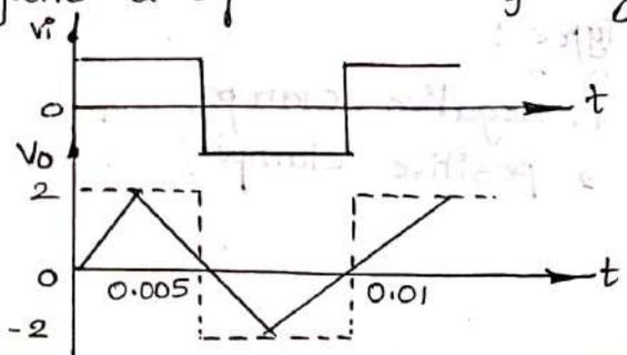
3. Sketch the output waveforms of a differentiating circuit with square wave input for  $R_C = \rho \omega$  and  $R_C = \rho \omega / 10$ .
