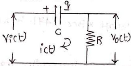
The dia. shows high pass RC circuit.
