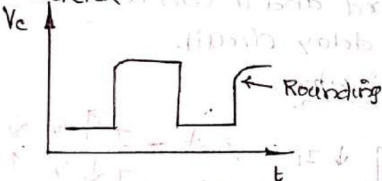
There is a certain distortion present in the output as a square wave of collector coupled Astable multivibrator is called rounding.
