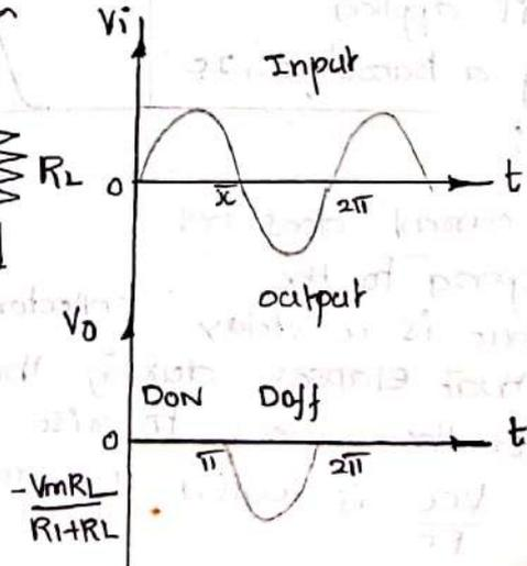
6. Parallel clipper with Voltage divider:
