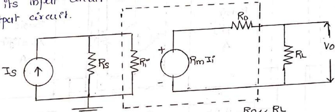
In this amplifier, an output voltage is proportional to the input signal current and the proportionality factor is independent on the source and load resistance.
