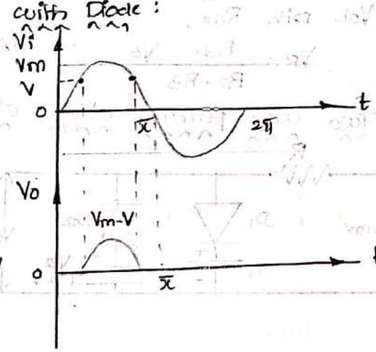
→  $V_i > V$  start conduction  $V_o = V_i - V$
