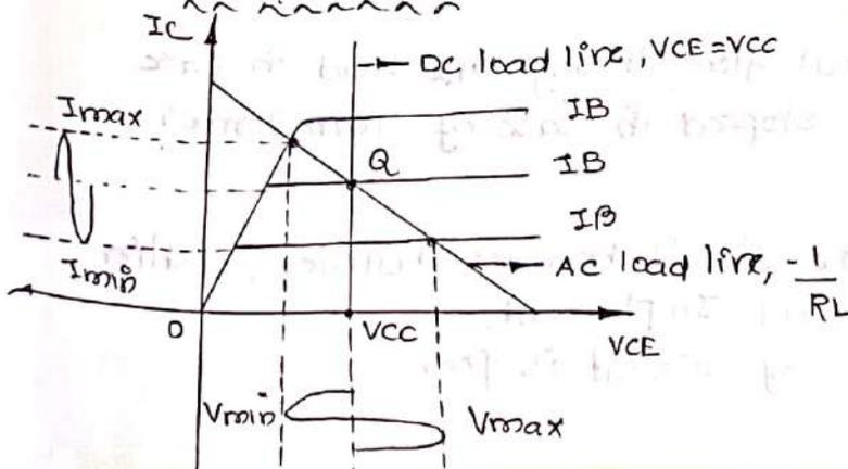
For ac purpose, the secondary is  $R_L$  and primary is  $R_L'$ . So ac load line is  $-1/R_L$  slope passing through Q-point. When ac input is applied the  $I_C$  varies around its Q value  $I_{CQ}$  and also output voltage varies sinusoidally around its Q-value  $V_{CEQ}$  which is  $V_{CC}$  in case.
