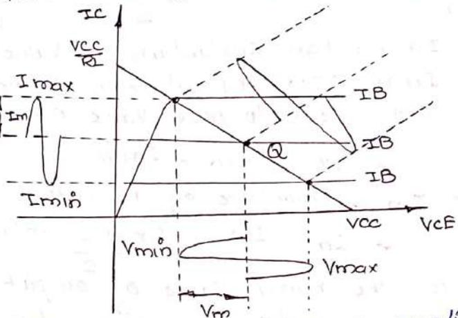
A Fixed Bias circuit can be used as class A amplifier. The value of  $R_B$  is selected in such a way that Q-point lies at the centre of dc load line. Here  $R_L$  is directly connected in collector circuit.
