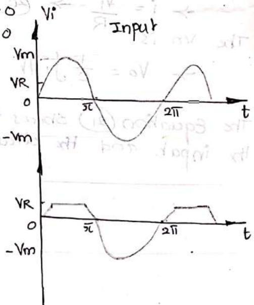
$$V_o = V_i \quad \text{for } V_i < V_R$$
