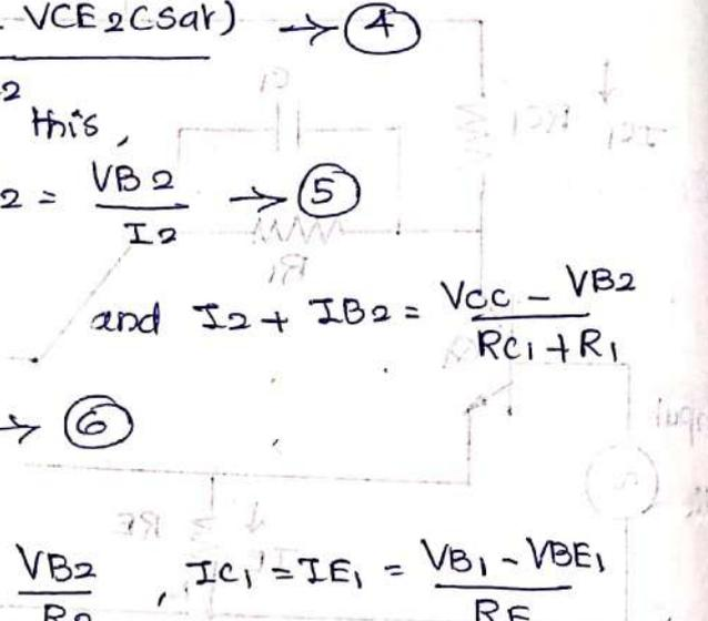
$$\text{cont. } I_{B2} = \frac{V_{CC} - V_{BE(\text{sat})}}{R} = 15 \mu = \frac{10 - 0.7}{R}$$
