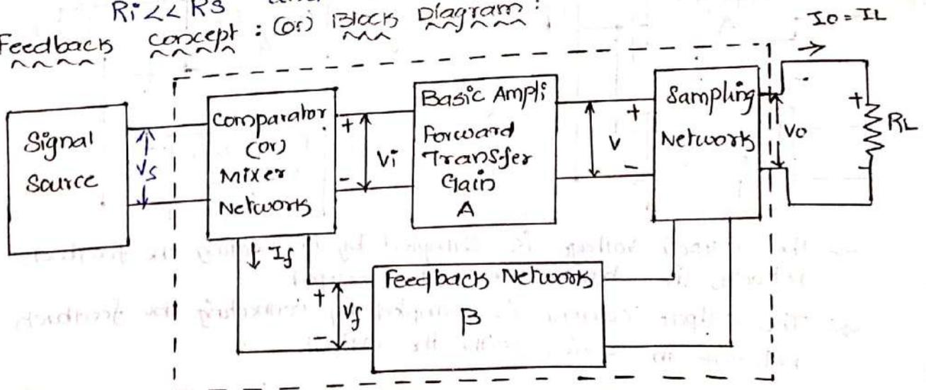
We can sample the output voltage or current by means of suitable sampling networks and apply this signal to the input through a feedback two port networks.
