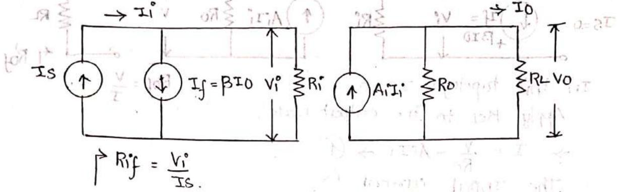
The above diagram, the amplifier input circuit is Norton's Model and output circuit is also Norton's Model.
