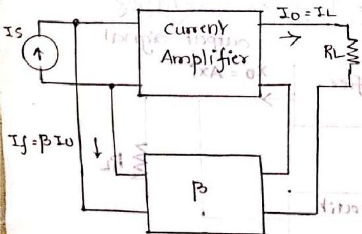
4. Transresistance amplifier with voltage shunt feedback:
