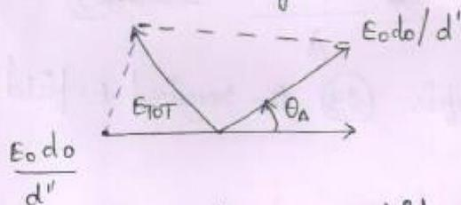
Referring to the phasor diagram which shows how the direct and ground reflected wave combines the electric field (at the receiver) at a distance  $d$  from the transmitter can be written as
