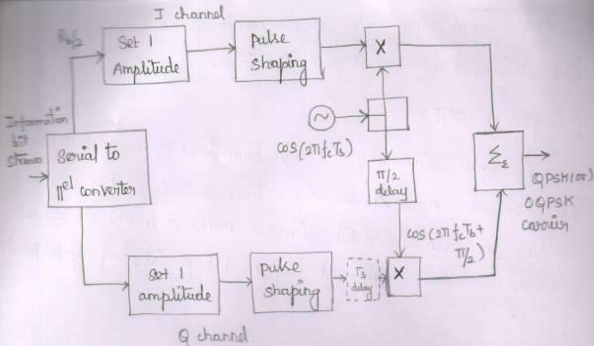
The result of this sample change is that phase shifts at any one time are limited & hence offset QPSK is more constant-envelope than straight QPSK.
