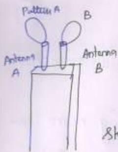
The mutual coupling which depicts that antenna B acts as reflector for antenna A, whose pattern is skewed to left. By the by Antenna B pattern is skewed to right due to reflections from antenna A.
