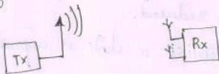
Single input multiple output means that the receiver has multiple antennas while the transmitter has one antenna.
