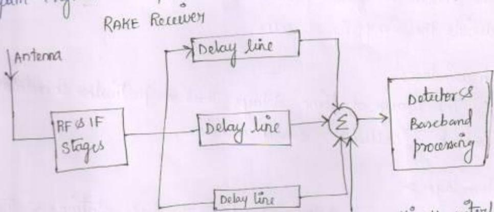
One of the advantage of CDMA system is the multipath interference can be reduced by combining direct & reflected signal in the receiver. The receiver used are called RAKE receivers
