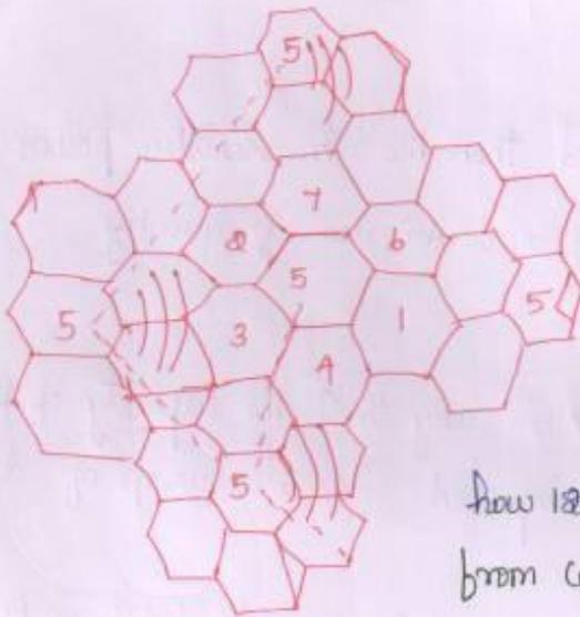
How  $120^\circ$  sectoring reduces interference from co-channel cells
