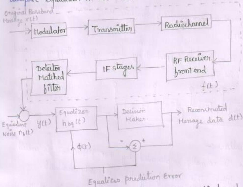
$f(t)$  = combined IR of transmitter multipath radio channel & receiver RF/IF
