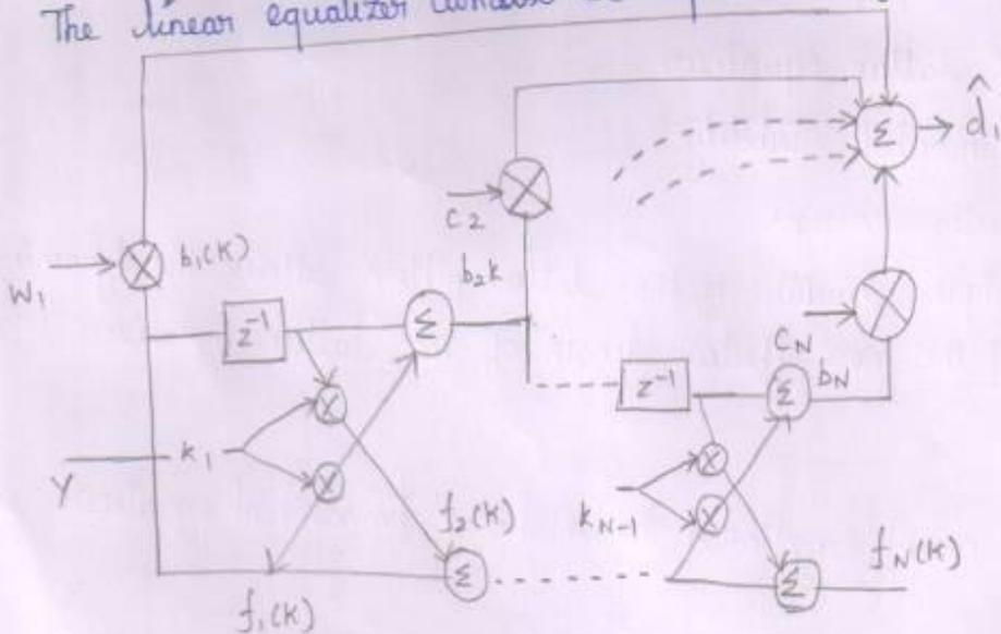
In this type of filter the i/p signal  $y_k$  is transformed into set of  $n$  intermediate forward & backward error signals  $f_n(k)$  &  $b_n(k)$  respectively
