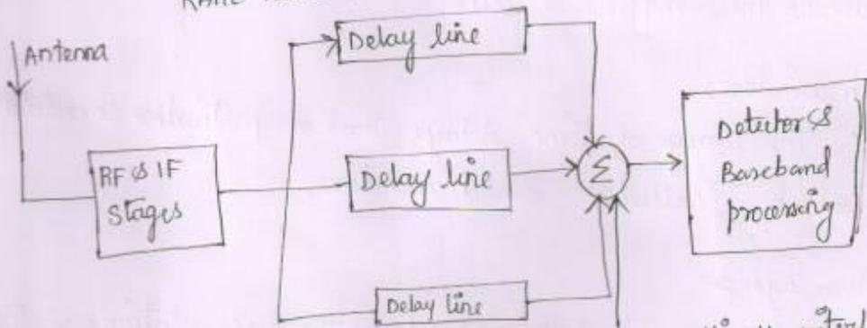
One of the advantage of CDMA system is the multipath interference can be reduced by combining direct & reflected signal in the receiver. The receiver used are called RAKE receivers
