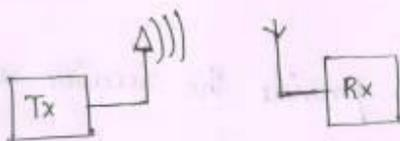
Single i/p single o/p means that the transmitter and receiver of the radio system have only one antenna.
