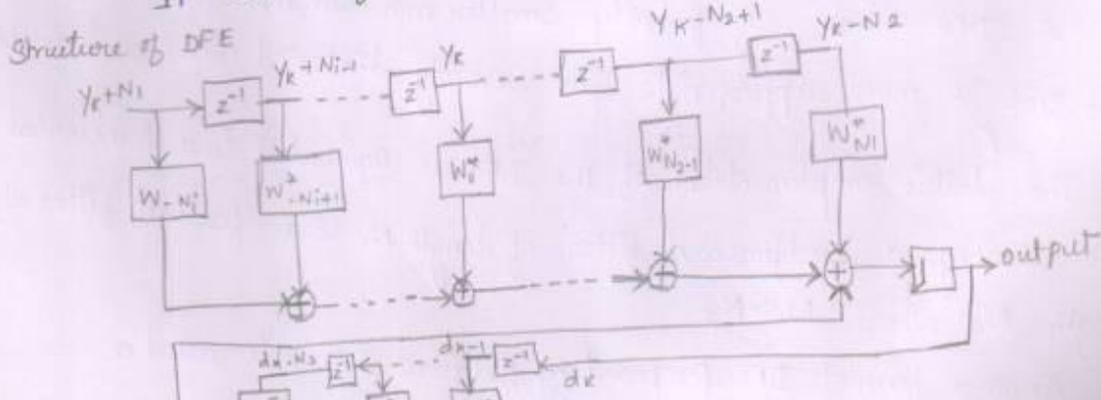
The FBF is driven by decisions on the o/p of the detector & its coefficients can be adjusted to cancel the ISI on the current symbol from past detected symbols.
