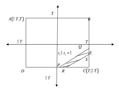
The double integral (1) is evaluated over the area of the square ABCD bounded by the  $t_1 = -T, T \& t_2 = -T, T$  as shown in the figure
